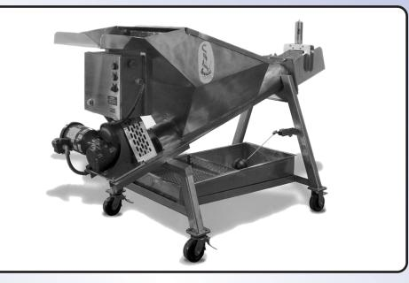
This unique machine ends forever the costly labor of manually separating liquid products from the containers for disposal or recycling. The Python Separator I opens, empties, and compacts the containers for disposal or recycling while effectively transporting the contents to a storage tank for removal.
